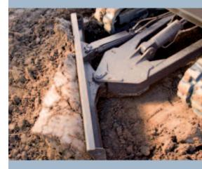
Hydraulic angle blade rotates to save time.
